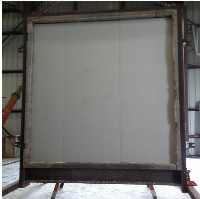
Photo No. 38 Completed base layer of GWB on unexposed face Exterior Exposure
