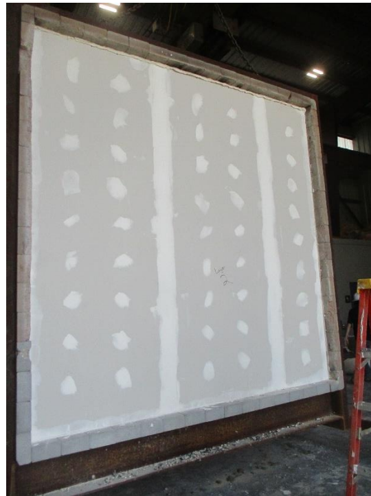
Photo No. 44 Completed Unexposed face - (Hose Stream Retest Assembly) Exterior Exposure
