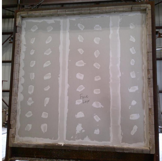
Photo No. 29 Completed face layer of GWB on unexposed face Exterior Exposure
