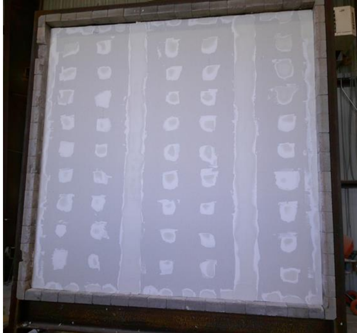
Photo No. 3 Completed face layer of GWB on exposed face Interior Exposure
