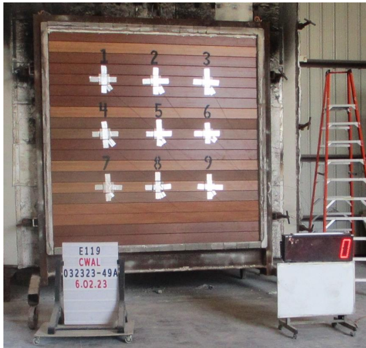
Photo No. 14 Completed Test Set-Up – (Interior Exposure Pre-Test)
