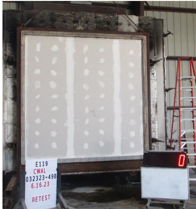
Photo No. 49 Exterior Exposure - Completed Hose Stream Retest Set-up
