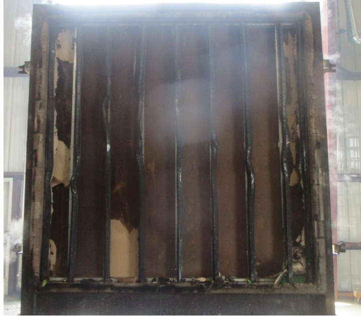
Photo No. 53 Exterior Exposure - Exposed Face – (Post-Hose Stream Retest Application)
