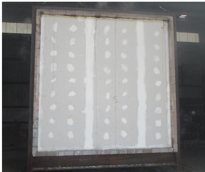
Photo No. 52 Exterior Exposure - Unexposed Face – (Post-Hose Stream Retest Application)
