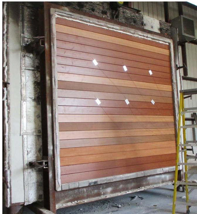
Photo No. 12 Completed installation of ChamClad 6-in. wide, V-groove PVC exterior panels (Unexposed Face) Interior Exposure
