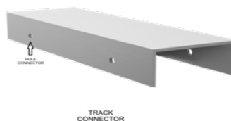
Quick Click Aluminum Track Connector 4.7" (119mm) Length 1.38" (35mm) Width 0.6" (15.24mm) Height
