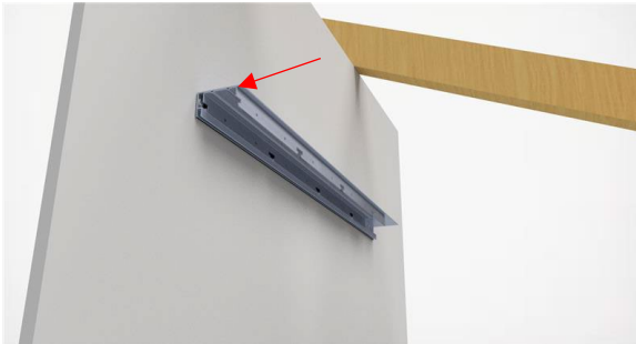
Example of Option 1 with base trim and track
