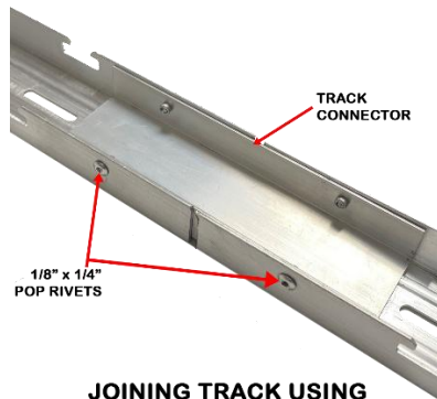
JOINING TRACK USING TRACK CONNECTOR
